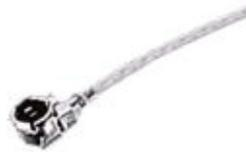
Figure 2.37: UFL antenna connector
