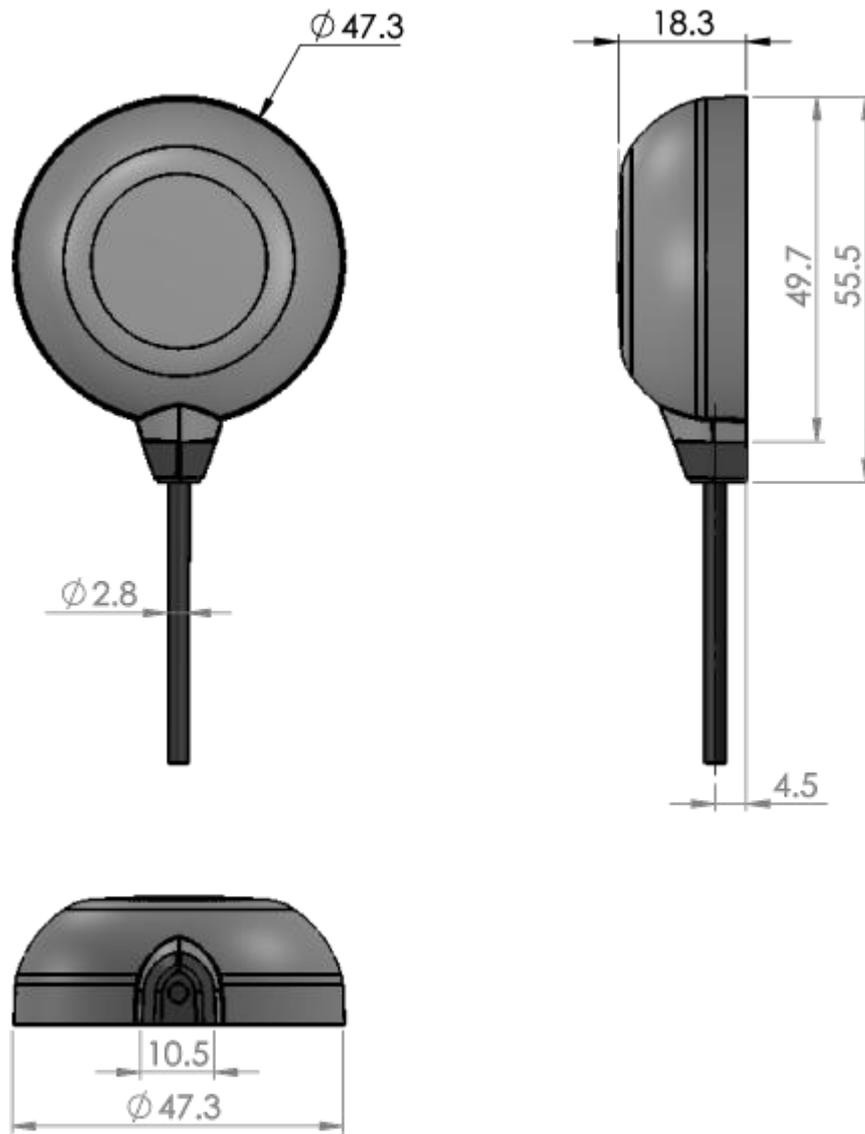
Figure 5.11: Tallysman 33-7882-07 mechanical drawing
