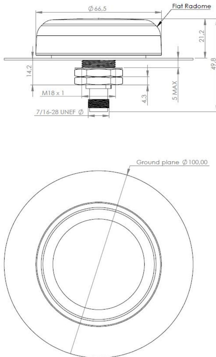
Figure 5.15: Tallysman TW3972 mechanical drawing
