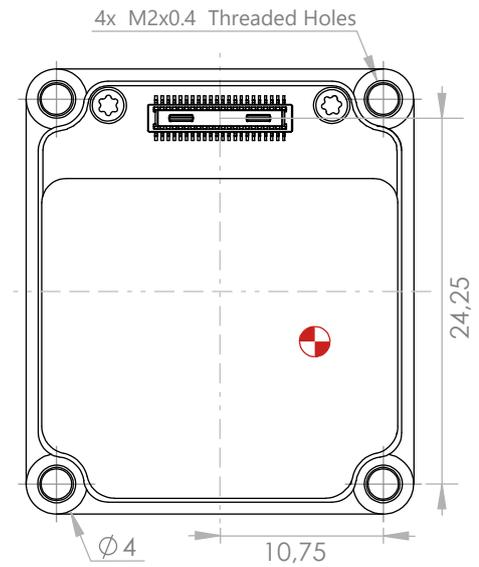
Figure 2.32: Ellipse-D Bottom view
