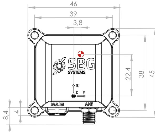
Figure 2.15: Ellipse-D top view
