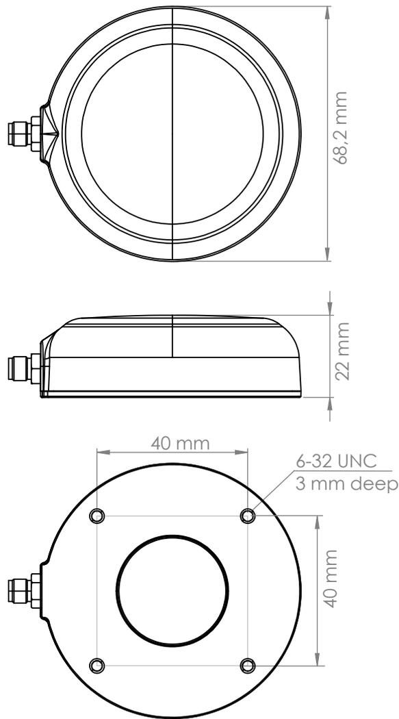
Figure 5.13: Tallysman 7972 mechanical drawing
