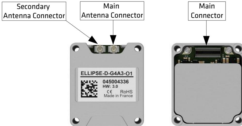
Figure 2.35: Ellipse INS with dual antenna GNSS receiver (OEM version)
