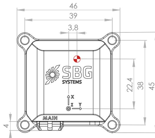
Figure 2.3: Ellipse-A top view
