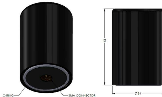
Figure 5.17: Maxtena M7HCT-A-SMA antenna mechanical layout. dimensions are in mm
