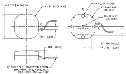
Figure 5.15: Antcom G5 antenna mechanical layout. dimensions are in inches [mm]
