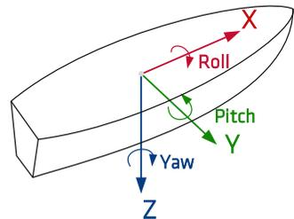
The Ellipse **MUST** be mechanically aligned with the vehicle coordinate frame, as explained in the following diagram.
