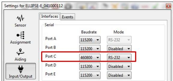
**Note:** Post Processing messages contain a lot of packets, sufficient baudrate speed should be then selected. We recommend a speed of 460 800 bps in that case.
