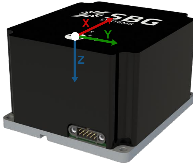
Figure 4.1: Quanta Extra IMU coordinate frame
